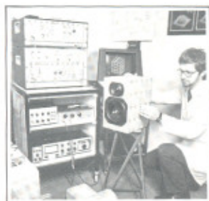
Employing the point accelerometer for measurement of vibration amplitude.
