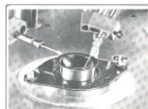
FFT2 tweeter construction employs automated assembly operations.
